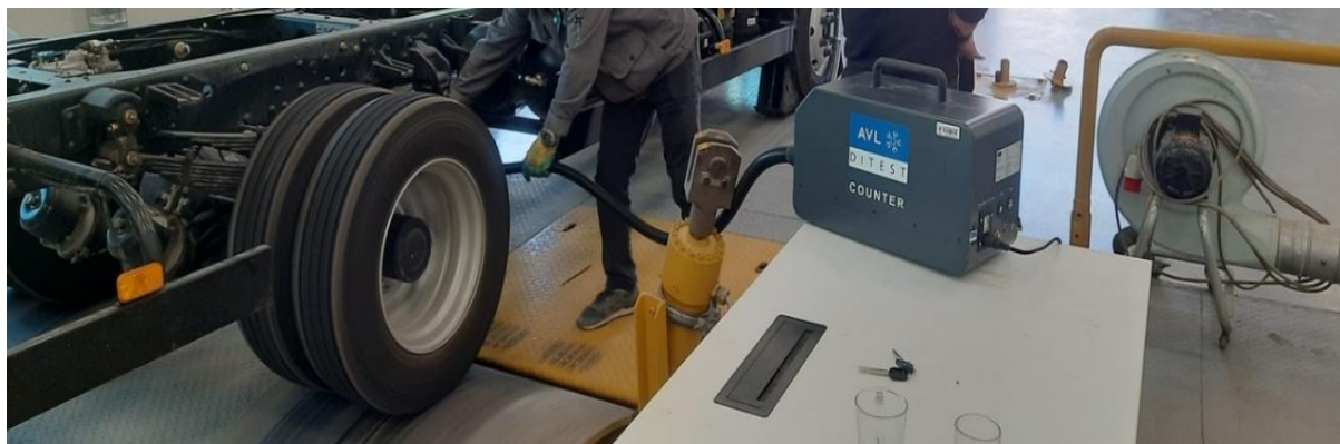
Figure 3: Device for measuring emitted particulate matter
